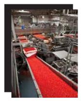
The tomatoes are hand sorted once agian and placed into different can sizes ranging from six ounces all the way to #10 cans (gallons).
