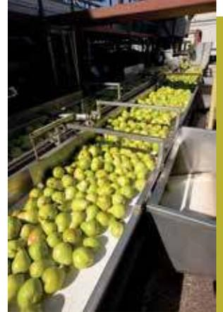
After sizing, the peaches are sent through the pitting machine, then dropped onto the conveyor where the Optical Color Sorter detects pits and defects with high speed cameras. Following machine inspection, the peaches and pears are examined by plant employees.
