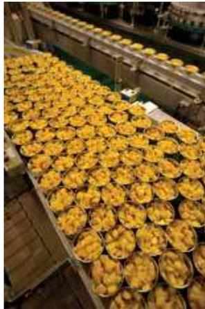
Some of the fruit is sent to our state of the art cold fill fruit bowl lines. The cups of fruit are cooked and sealed to lock in the nutrients.
