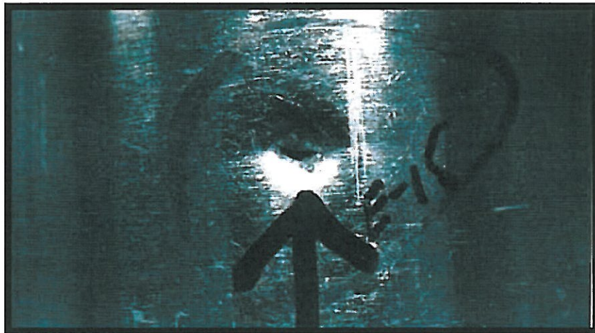
Photo 6: Puncture in can body. Pinholes in can body plate also cause loss of hermetic seal.
