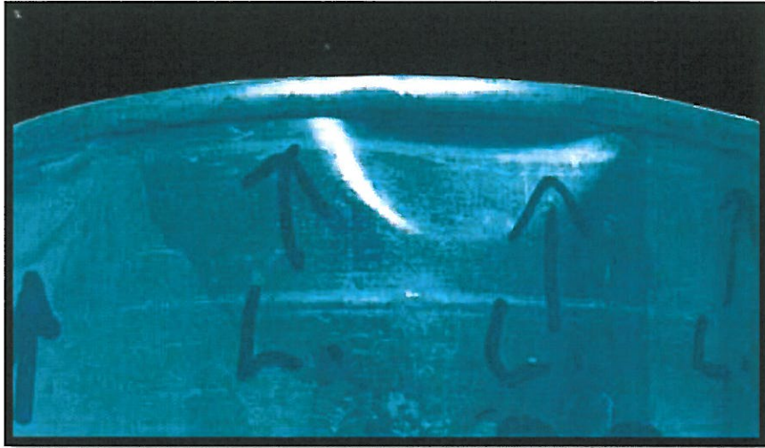
Photo 3: An opening below the double seam or plate fracture.
